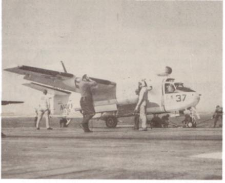
The S-2D Tracker is equipped with Magnetic Anomaly Detection gear which detects variations in the earth's magnetic fields induced by the presence of submarines.
