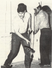
(above) Centerline anchor let go after a quick swipe at the limiting pelican hook with a sledge hammer...
